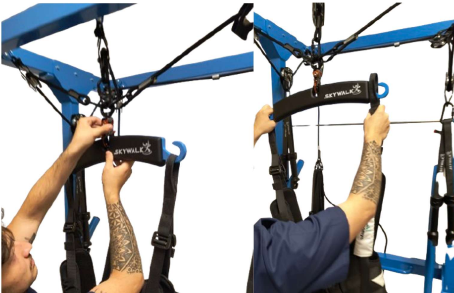
Figure 4: Attachment of the hanger bar (Left) and attachment of the harness on the hanger bar (Right)
